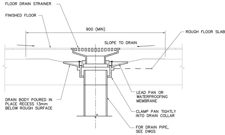
2 ROOF DRAIN (RD-2) DETAIL
