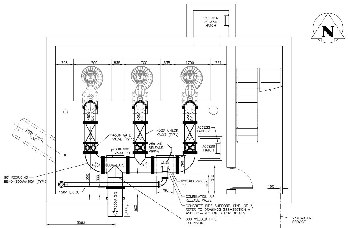
MECHANICAL FLOOR PLAN
