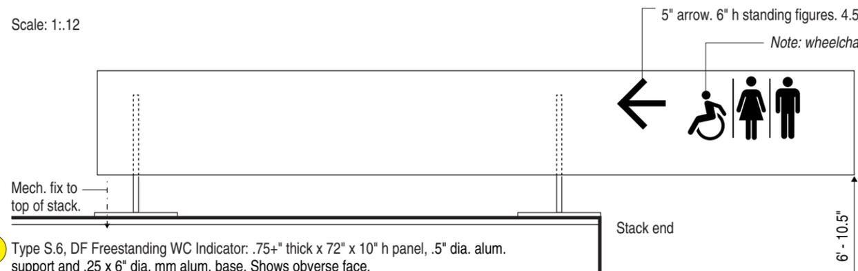
**.\_21** Type S.6, DF Freestanding WC Indicator: .75+ inch thick x 72 inch x 10 inch h panel, .5 inch dia. alum. support and .25 x 6 inch dia. mm alum. base. Shows obverse face.
