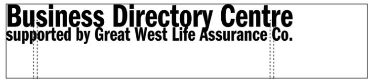
**.\_20** Type S.4, DF Freestanding Stack Indicator: .75+ inch thick x 48 inch x 10 inch h panel, .5 inch dia. alum. support and .25 x 6 inch dia. mm alum. base. Note messages flush left or right to stack end. Shows obverse face.
