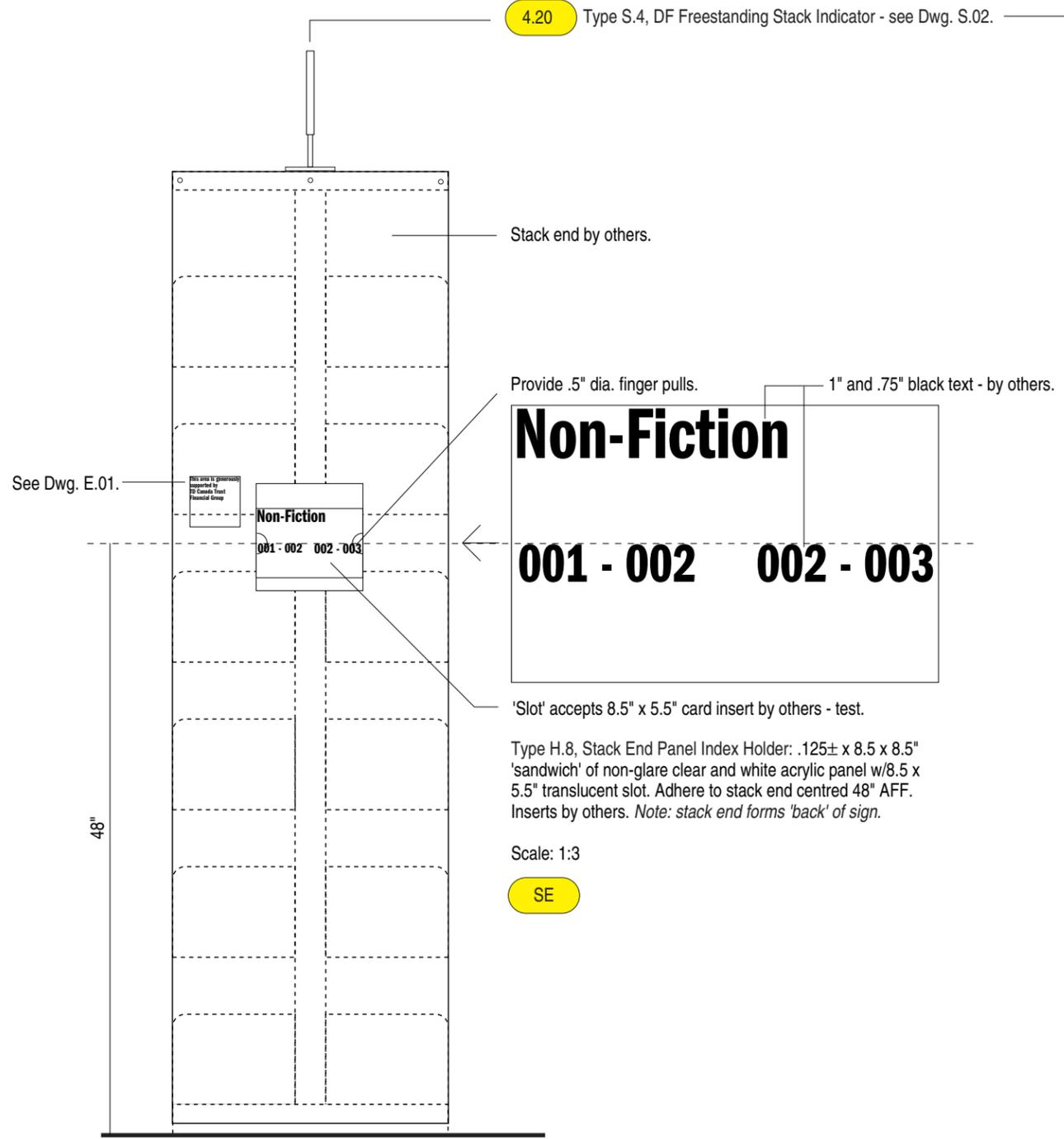
Level 4; stack end elevation.
