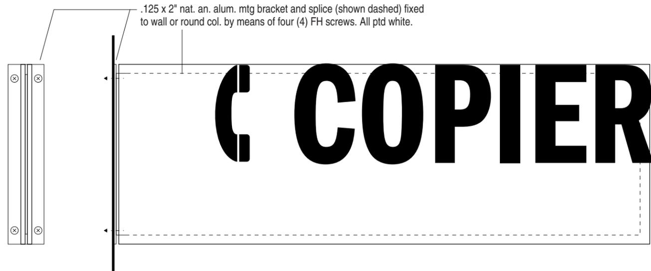
.125 x 2" nat. an. alum. mtg bracket and splice (shown dashed) fixed to wall or round col. by means of four (4) FH screws. All ptd white.
