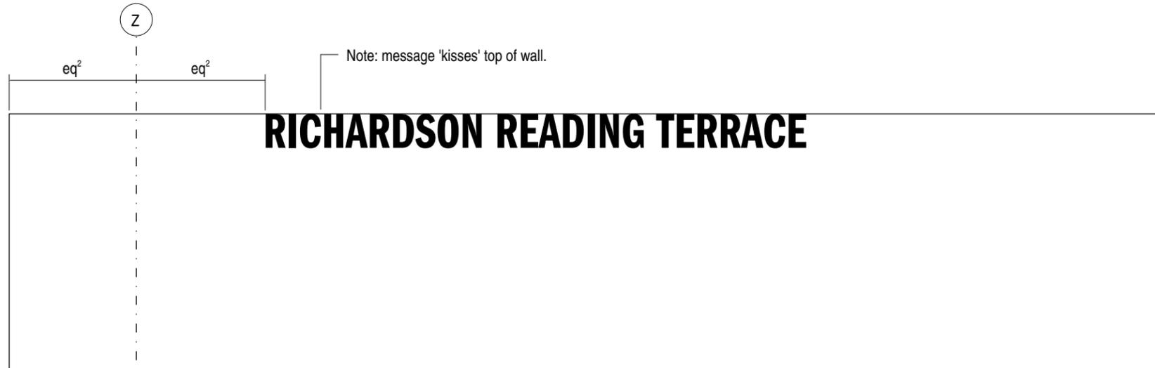
**1.35** Type L.6: .1875" x 6" h nat. anod. alum. letters pin-mounted onto wood wall. Location t.b.site c. .5" = 12"
