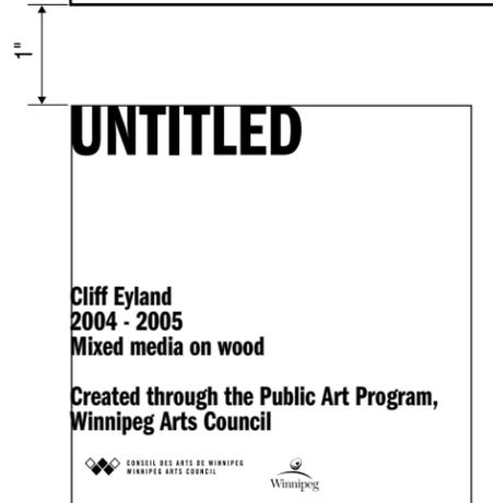
**S1** Type M.4: .1875" x 4 x 4" nat. anod. alum. plaque w/engraved and infilled (matte black) text. *Note location relative to work - site confirmed.*
