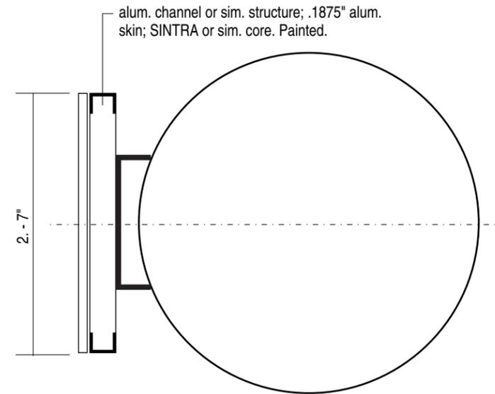
Type K.10, plan view. Invisibly bracket sign approx. 1" off 31.5" dia. conc. col. by means of 2" x 12" x 93" alum. channel.
