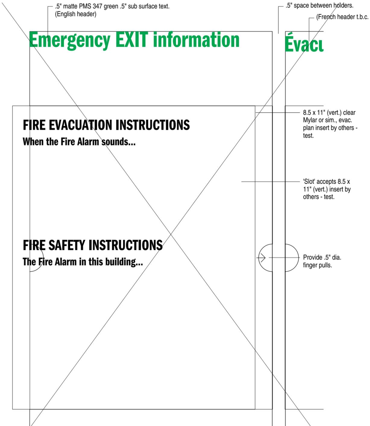
**3** Type H.9 (Evac. Plan Holder): .25± x 8.5" x 14.35" non-glare clear acrylic w/rev. sub surface text, slot, VHB adhesive. Centre on wall or sidelite 2" from door frame (or as site instructed), 48" AFF. Note: consists of two (2) holders, one (1) Eng., one (1) Fr.
