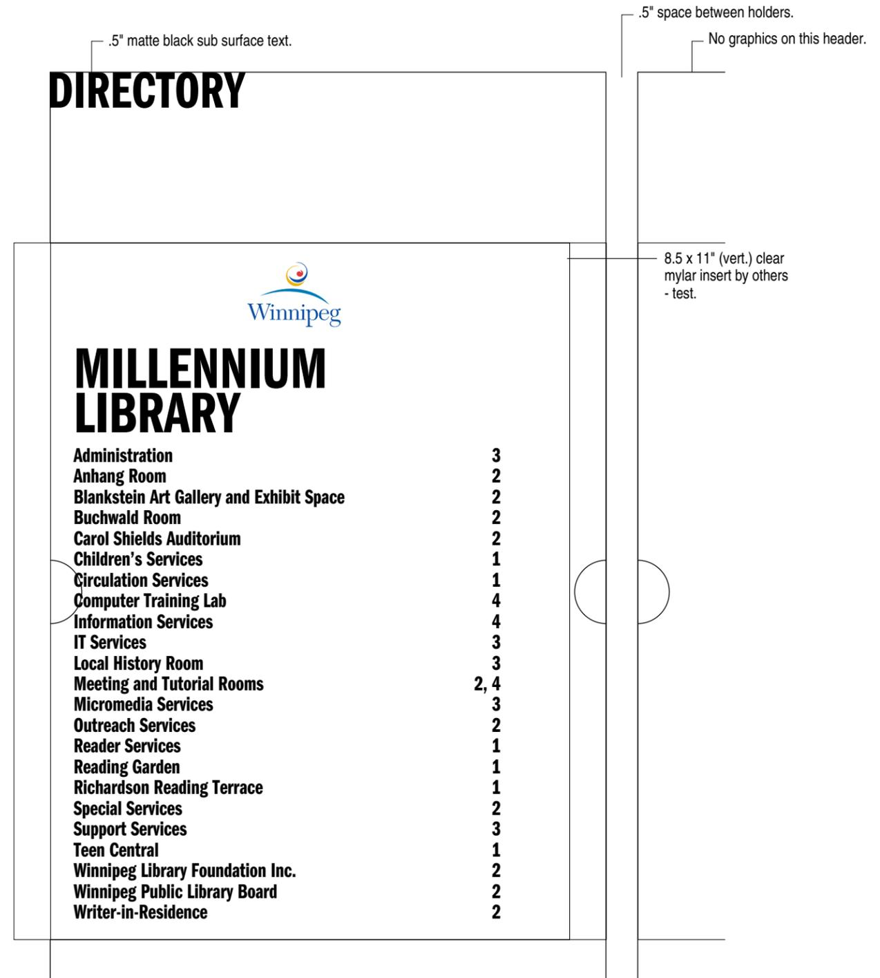
**V** Type H.9 (Elevator Directory Holder): .25± x 8.5" x 14.35" non-glare clear acrylic w/rev. sub surface text, slot, VHB adhesive. Centre on glass wall between elevator frames (or as site instructed), 48" AFF. 2 signs side by side req'd in each location.
