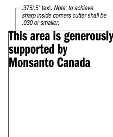
**PL.3** .1875" x 4 x 4" lamacoid plaque w/engraved and infilled or silkscreened (matte black) text. Stack end-mounted centred 48" AFF or as site instructed.
