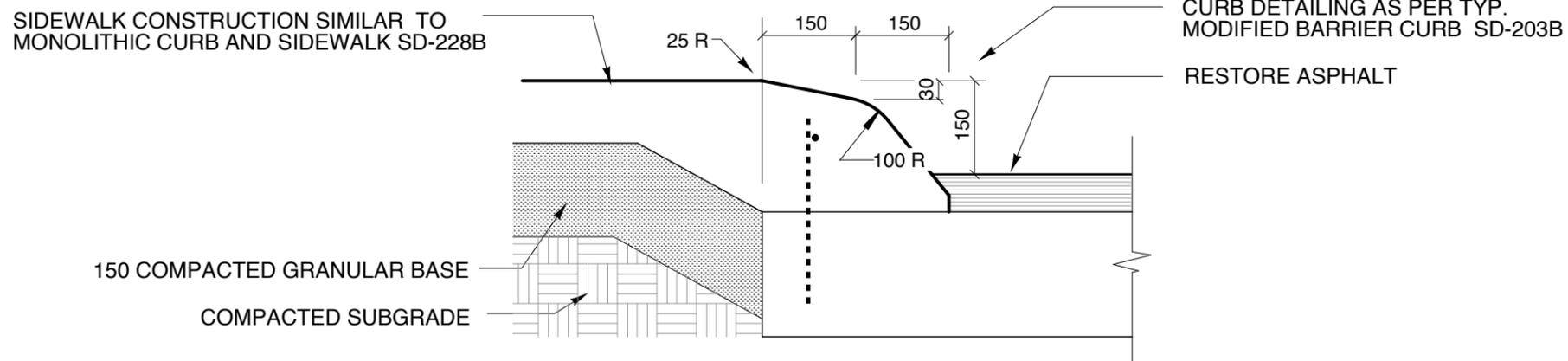
NOTE: USE THIS CURB PROFILE AT ALL INTERSECTION CURVES AS PER STANDARD LAYOUT SD-229A
