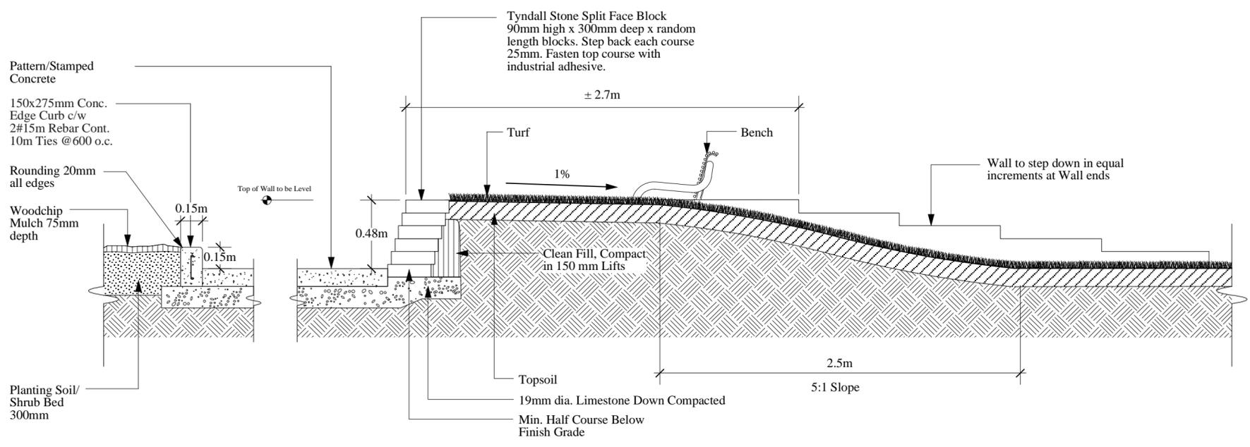
**2** Slope Section with Tyndall Stone Wall and Edge Curb
