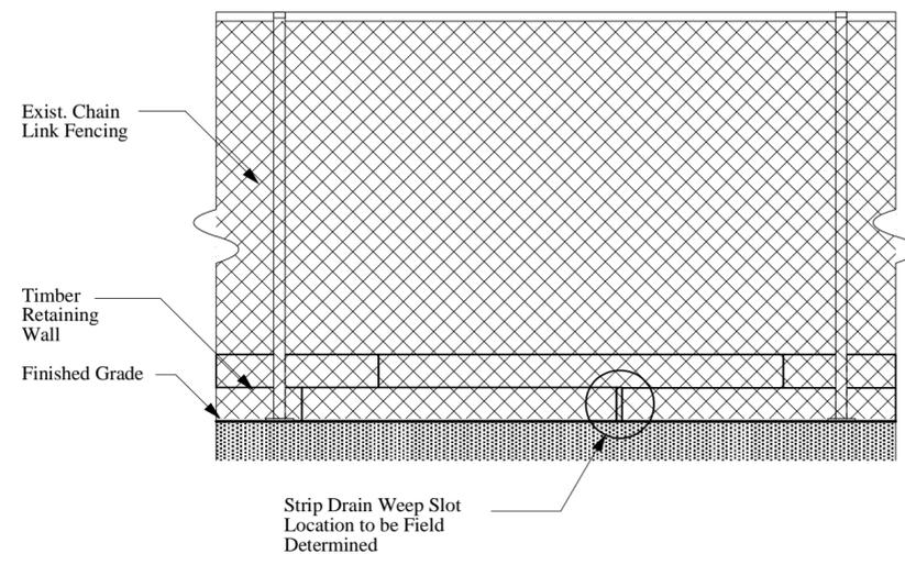
5 East or West Streetside Retaining Wall Elevation
