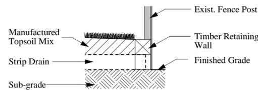
2 Strip Drain Weep Slot Section
