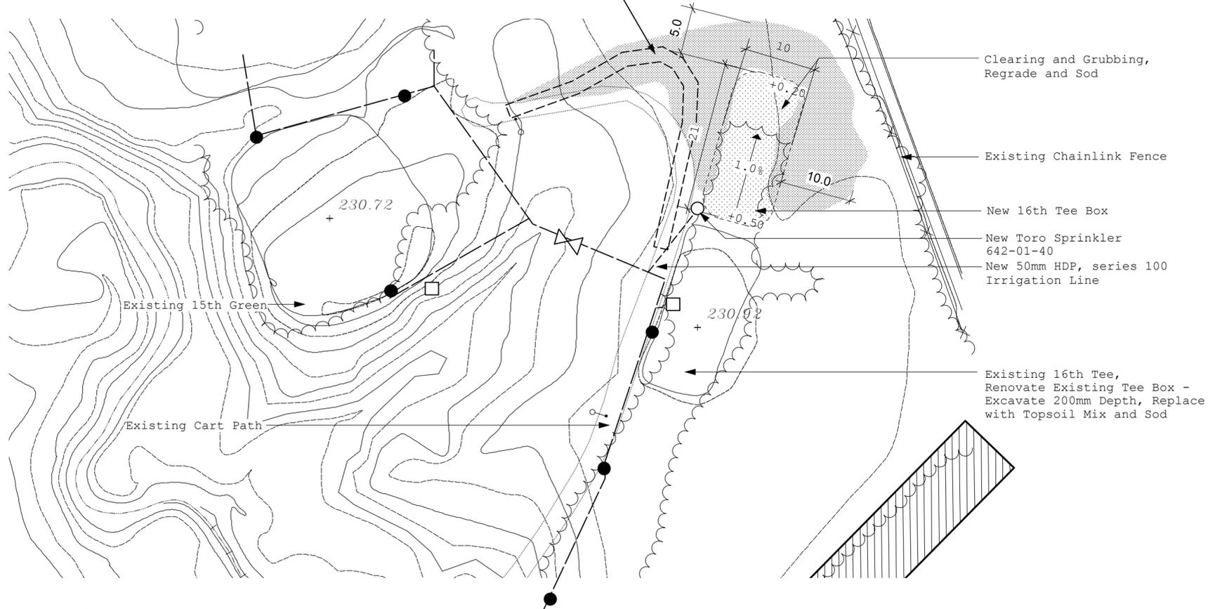
**2 Grading and Layout Plan - 16th Tee Box Expansion and Renovation**
