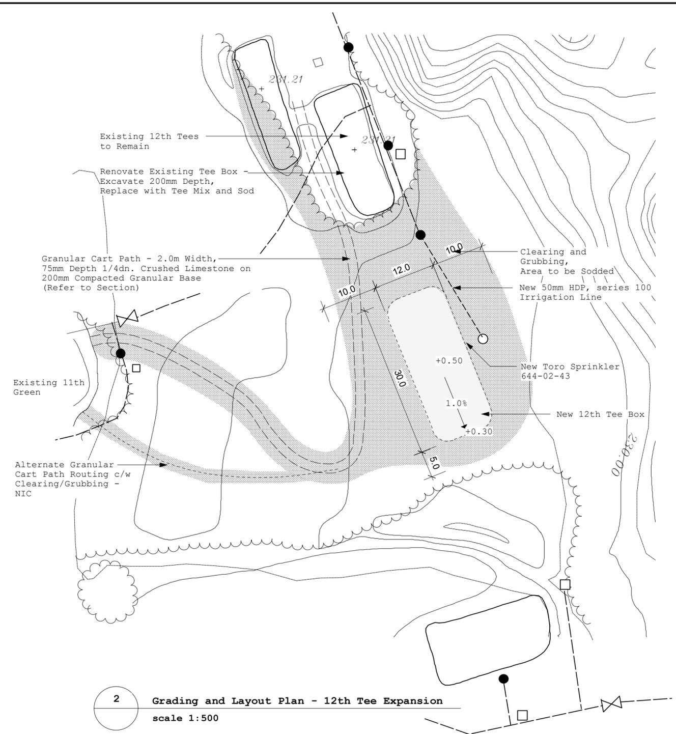
2 Grading and Layout Plan - 12th Tee Expansion
