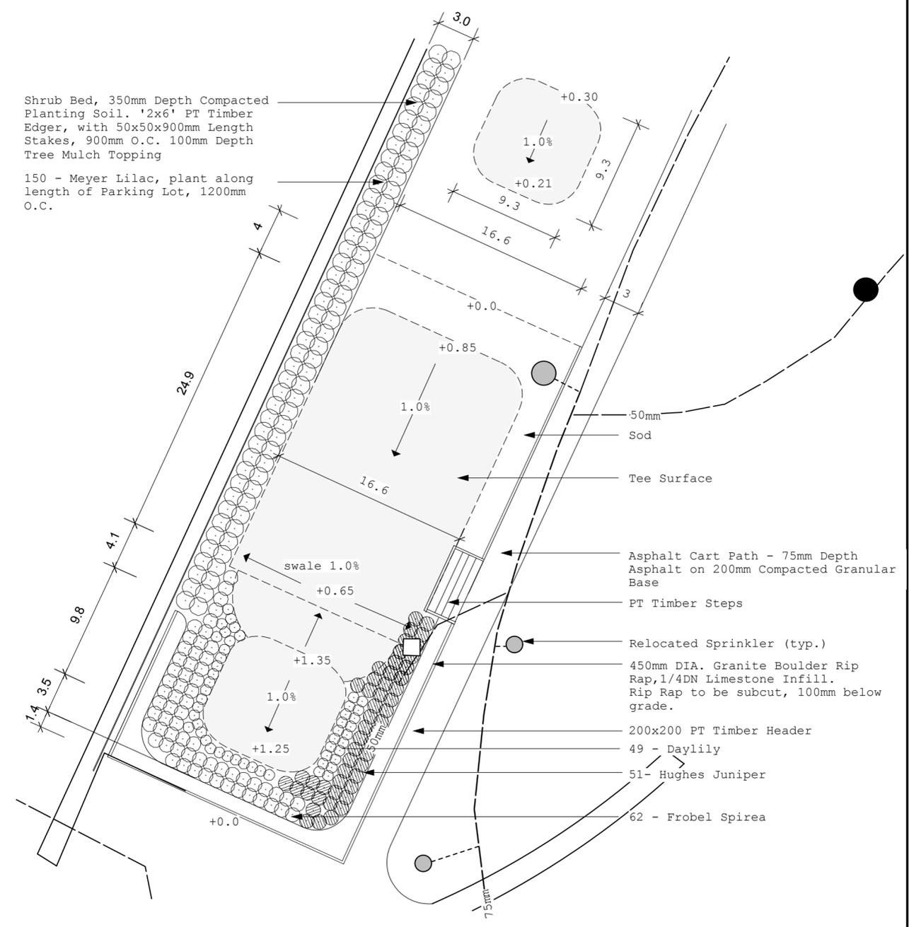
**3 Grading and Layout Plan - Two-Tiered Tee Box Expansion**
